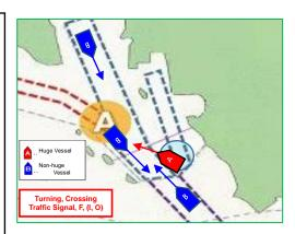
A. When a huge vessel departs to shift, via the Inner Harbor Passage, and enters the Turning Basin.
